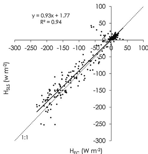
Fig. 7. The correlation between the sensible heat fluxes measured by the eddy covariance ( $H_{EC}$ ), and the surface layer scintillometer ( $H_{SLS}$ ); the solid line is the linear regression line, and the dash line is a 1:1 line.
