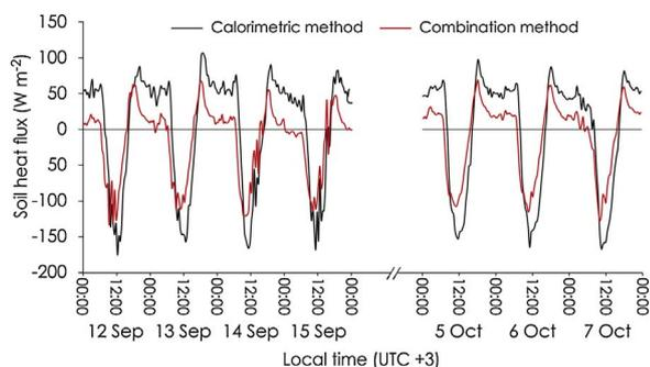
Fig. 5. 30 min average of the soil heat flux computed by the calorimetric method and by the combination method.
