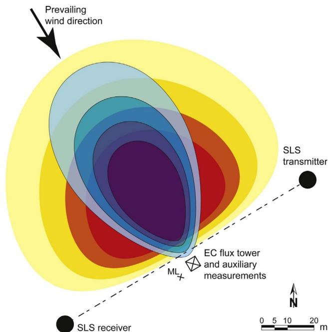
Fig. 2. Top view of the experiment design. The transmitter and receiver of the surface layer scintillometer (SLS) are placed at a distance of 100 m. The eddy covariance (EC) flux tower, microlysimeter, and complementary meteorological measurements are placed in the middle of the SLS path. The approximated footprints of SLS and EC are illustrated by warm and cold colors for the SLS and EC, respectively. Increase in hue saturation indicates greater contribution to the measured flux.
