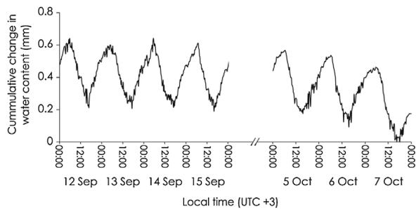
Fig. 8. Cumulative change in water content. Changes were determined relative to the lowest mass point, which was set at zero.
