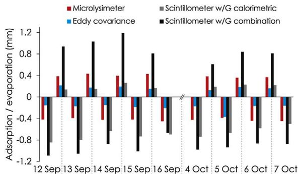
Fig. 9. Daily total adsorption (positive) and evaporation (negative) measured by the different methods.
