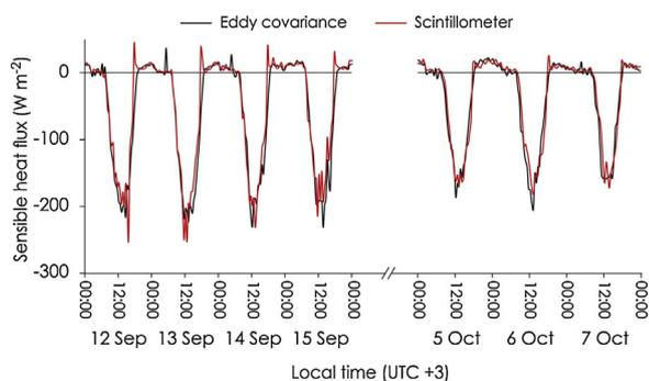
Fig. 6. 30 min average of sensible heat flux measured with eddy covariance and the surface layer scintillometer.
