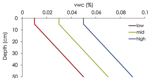
Fig. 3. Values of volumetric water content (VWC) profile used for the sensitivity analysis of soil heat flux calculations. The predetermined profile is in green (mid); Red and blue are 2% lower (low) and higher (high) VWC value, respectively. (For interpretation of the references to colour in this figure legend, the reader is referred to the web version of this article.)
