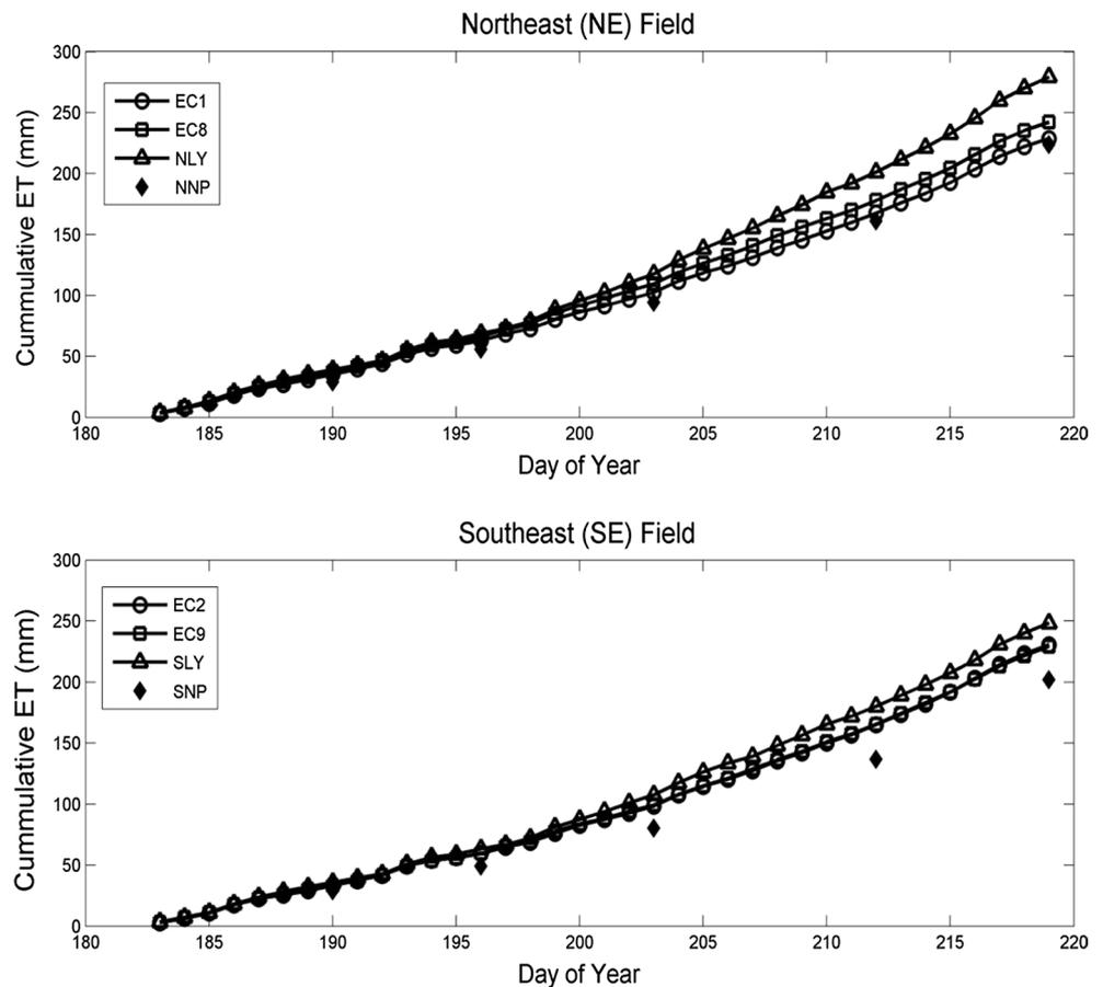
**Table 1** The cumulative ET over the whole of the study period (DOY 183–220) is shown for each measurement technique for both the NE and SE fields
