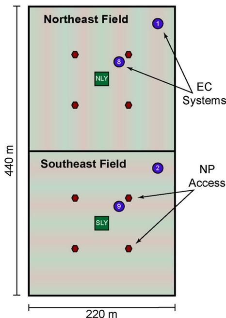
**Fig. 1** Schematic showing the location of the eddy covariance systems (EC sites 1, 2, 8, and 9), stations, lysimeters (NLY and SLY), and the network of neutron probe sensors (NNP and SNP) in the northeast (NE) and southeast (SE) fields
