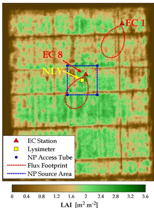
**Fig. 3** The typical source area (flux footprint) for the EC towers in the NE field (EC1 and EC8) along with the source area for the NE lysimeter (NLY) and NE neutron probe network (NNP) network are shown overlaying the LAI map from DOY 202
