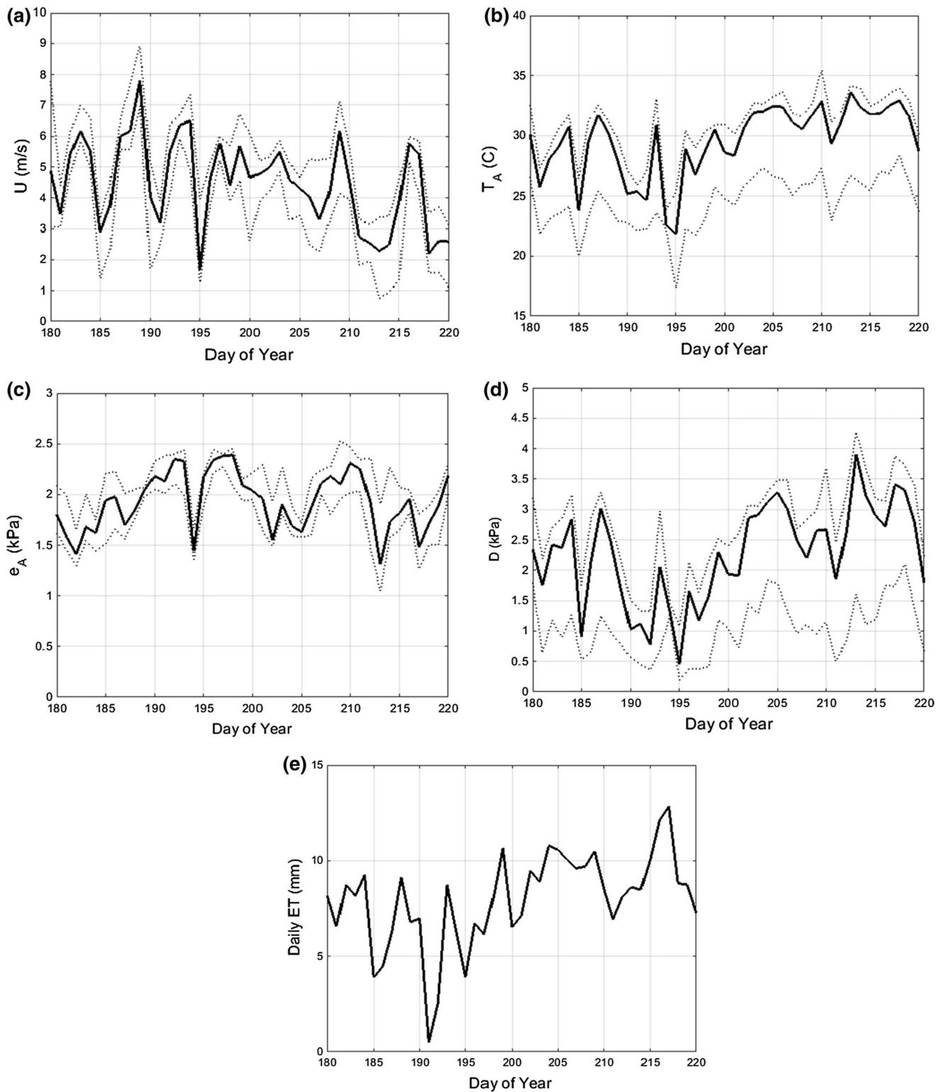
**Fig. 2** Median (solid line) and max/min (dotted lines) of **a** wind speed ( $u$ ), **b** air temperature ( $T_A$ ), **c** vapor pressure ( $e_A$ ), and **d** vapor pressure deficit ( $D$ ) from the four EC systems in the NE and SE
