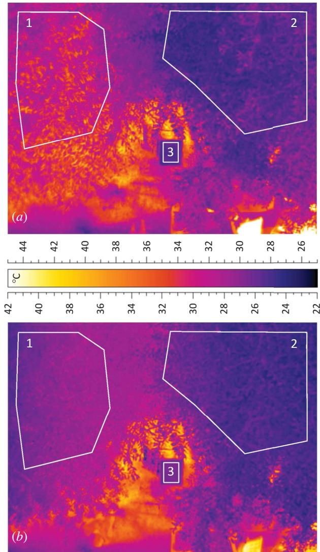
Figure 2. Example of 1 min thermal images extracted from the video recording. (a) Filmed at 10:10 (solar radiation  $\sim 720 \text{ W m}^{-2}$ ) and (b) filmed at 10:16 (solar radiation  $\sim 230 \text{ W m}^{-2}$ ). Polygons 1 (stressed) and 2 (well-watered) in both panels mark the area from which average temperatures were determined. Rectangle 3 marks the area used to determine the wet reference temperature.
