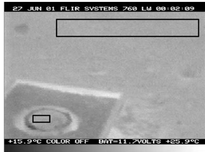
Figure 2. A sample of a thermal image of the microlysimeter and its surrounding, acquired at midnight 26–27 June. The gray level indicates the surface temperature (the brighter the color, the warmer the surface). The dark area around the soil sample is the polypropylene isolation. The two rectangles mark the subsets from which the pixels data were extracted.
