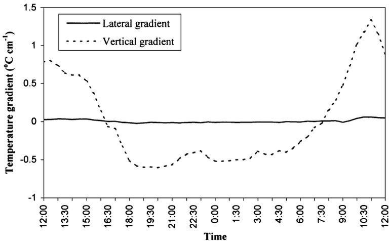
Fig. 4. Lateral and vertical temperature gradients inside the microlysimeter, measured at DOY 105–106, 2000 (first measurement period).
