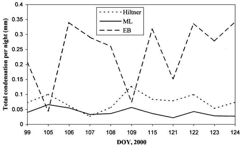
Fig. 2. Total condensation per night measured by the Hiltner dew balance (Hiltner) and the microlysimeter (ML) and calculated with the energy-balance equation (EB), for the first measurement period.
