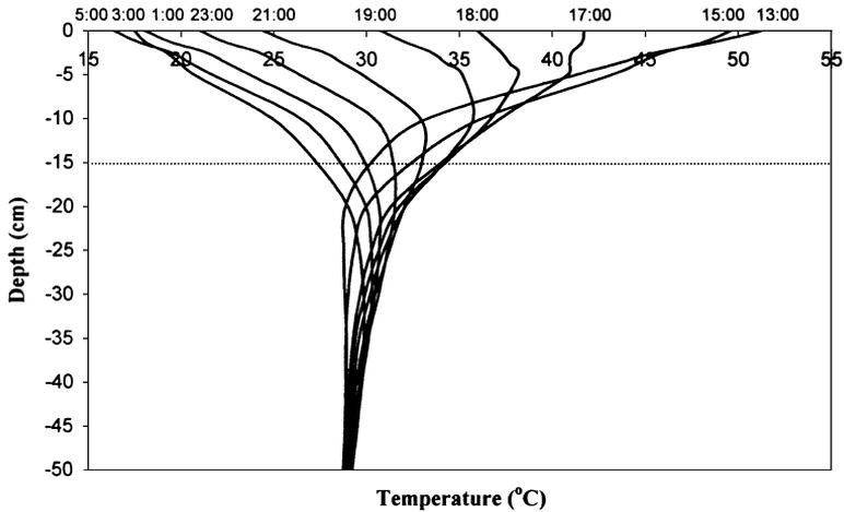
Fig. 5. Temperature profiles in the soil for different hours of the day, as measured on DOY 183, 2001 (beginning of the second measuring period).
