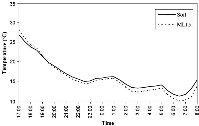
Fig. 3. Soil temperature at 1 cm depth inside (ML) and outside (Soil) the microlysimeter, for the 15 cm depth microlysimeter, measured at DOY 105–106, 2000 (first measurement period).
