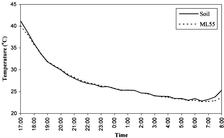
Fig. 7. Soil temperature at 1 cm depth inside (ML) and outside (Soil) the microlysimeter, for the ML<sub>55</sub>, measured at DOY 245–246, 2001 (second measurement period).
