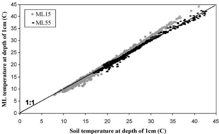
Fig. 8. Temperatures at 1 cm depth inside both ML<sub>15</sub> and ML<sub>55</sub> plotted versus the surrounding soil temperature at the same depth for all measured nights (from 17:00 to 8:00, every half hour).
