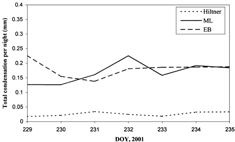
Fig. 9. Total condensation per night measured by the Hiltner dew balance (Hiltner) and the microlysimeter (ML) and calculated from the energy-balance equation (EB), for the second measurement period.
