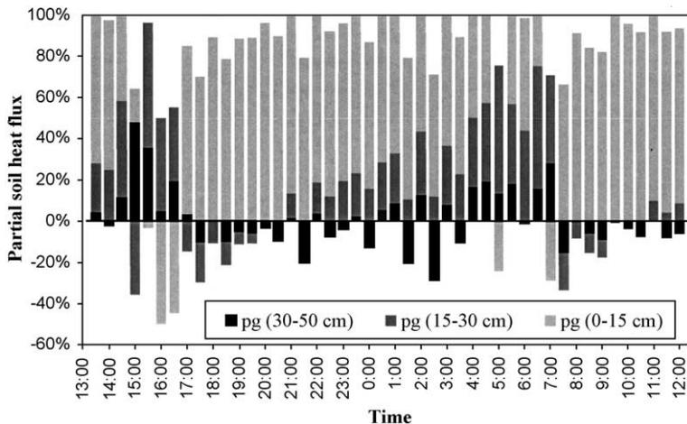
Fig. 6. Partial contribution of the different soil layers (pg 0–15, 15–30, 30–50 cm) to the total soil heat flux, for DOY 183, 2001 (second measurement period).
