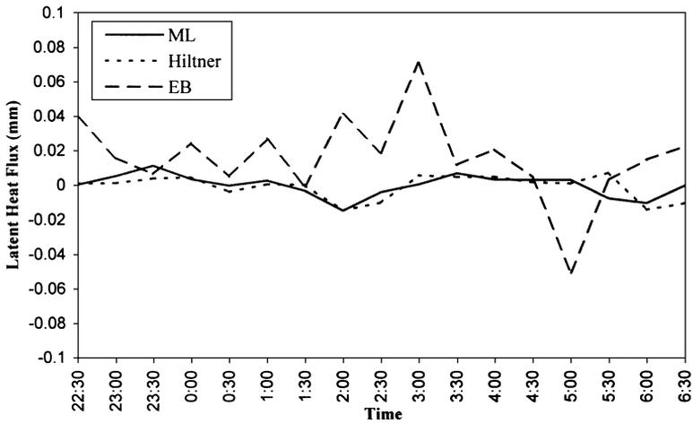
Fig. 1. Latent heat flux as measured by the Hiltner dew balance (Hiltner) and the microlysimeter (ML), and as calculated from the energy-balance equation (EB), for DOY 105–106, 2000, a representative day of the first measurement period.
